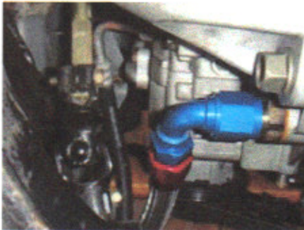
Connect oil line to adaptor installed on the engine front cover as shown.
