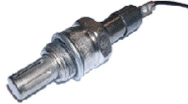
All petrol engined vehicles made for the UK market since 1993 have at least one Lambda sensor fitted. They are normally fitted into the exhaust manifold or down pipe of the vehicle in a position that is as close to the engine as possible. The body shape resembles that of a spark plug.
